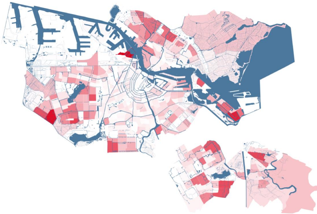
Figure 14 – Total watt peak from residential rooftop solar panels in 2024, grouped by neighbourhood
