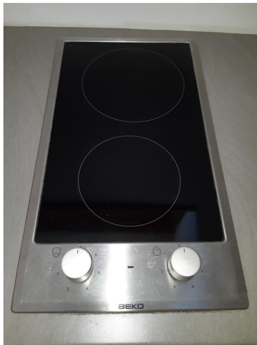
Figure 32: Ceramic hob of the brand BEKO, HDCC 32200 X, Class 1 used for the measurements of cooking processes as the power source was accessible
