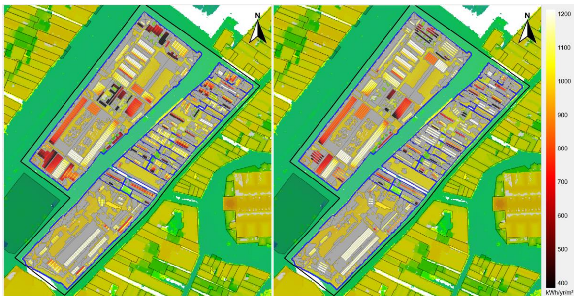
Figure 17 - Solar irradiation for solar modules for building groups in the focus district of the center of Amsterdam with east west-landscape (left) and south facing-portrait (right).
