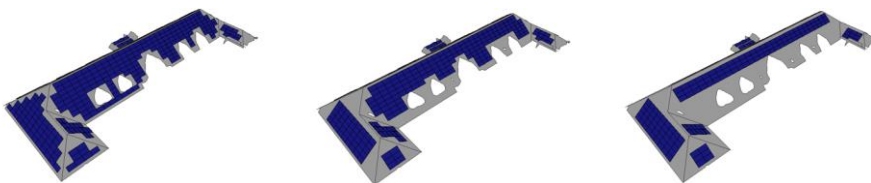
Figure 8 – Different choices of module layout methods. First the maximum possible on the left, then eroded in the middle and strictly rectangular on the right
